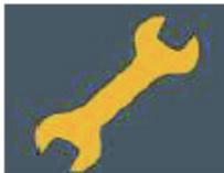
The yellow wrench symbol illuminates when the System Controller detects a mechanical, electrical, or software issue with the system.
