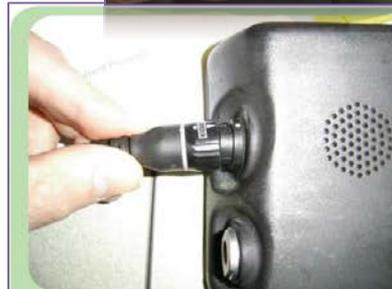
Correct for snap-lock and audible feedback
