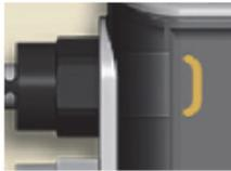
The yellow light near the black power cable connector illuminates when the black power cable becomes loose or disconnects from the System Controller.
