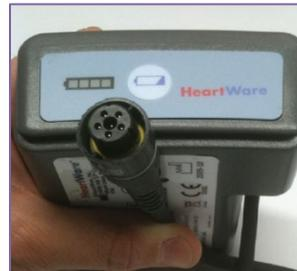
Power Source Connector with Pins
