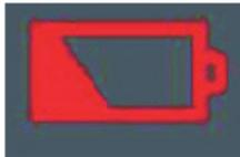
The red low battery symbol illuminates when less than 5 minutes of battery power remain (applicable only during 14 Volt Lithium-Ion battery-powered operation).
