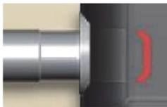
The red light near the driveline connector illuminates when the driveline becomes loose or disconnects from the System Controller.
