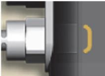
The yellow light near the white power cable connector illuminates when the white power cable becomes loose or disconnects from the System Controller.
